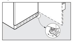
■ Use the flat wrench provided to adjust the feet as needed, so that the appliance is even all around.
